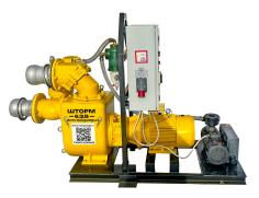
Common Characteristics: All pumps handle water with up to 10% abrasive content and particles up to 76 mm. The pump and impeller are made of cast iron, and steel compensating plates. The seal used is SiC/SiC/NBR. Inlet and outlet sizes are BRS DN 150 mm, and the maximum suction height is 8 meters.
