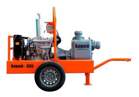
Common Characteristics: All pumps handle water with up to 10% abrasive content and particles up to 76 mm. The pump and impeller are made of cast iron, and steel compensating plates. The seal used is SiC/SiC/NBR. Inlet and outlet sizes are BRS DN 150 mm, and the maximum suction height is 8 meters.
